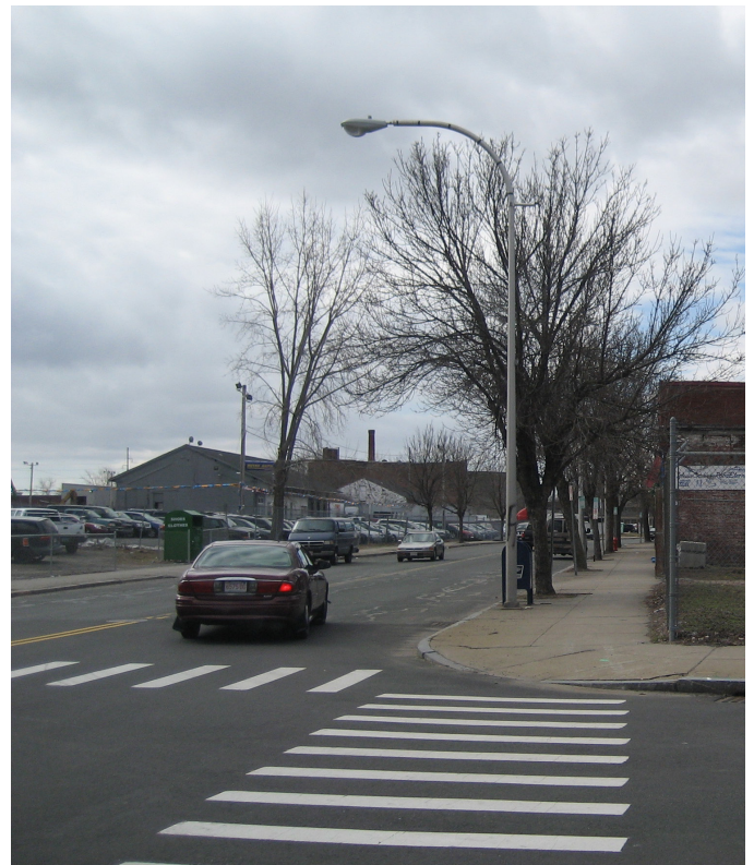
Trees along Main Street help to enhance the pedestrian environment. The cobra-head style lighting fixtures provide adequate light, but are scaled for cars rather than people.
