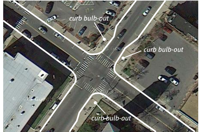
Curb bulb-outs at the intersection of Maple and Appleton Streets
